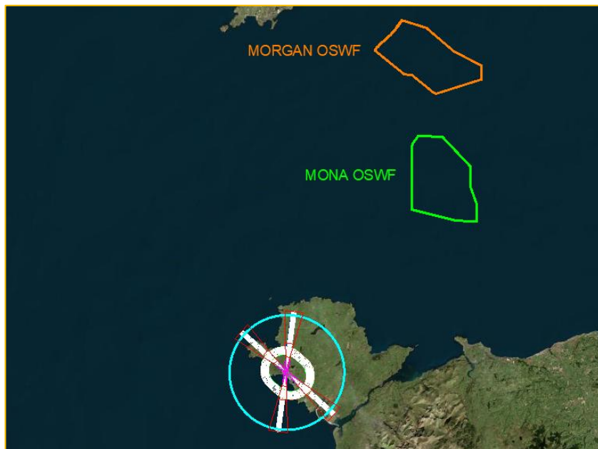
Figure 157 - RAF Valley OLS in Relation to Windfarms
